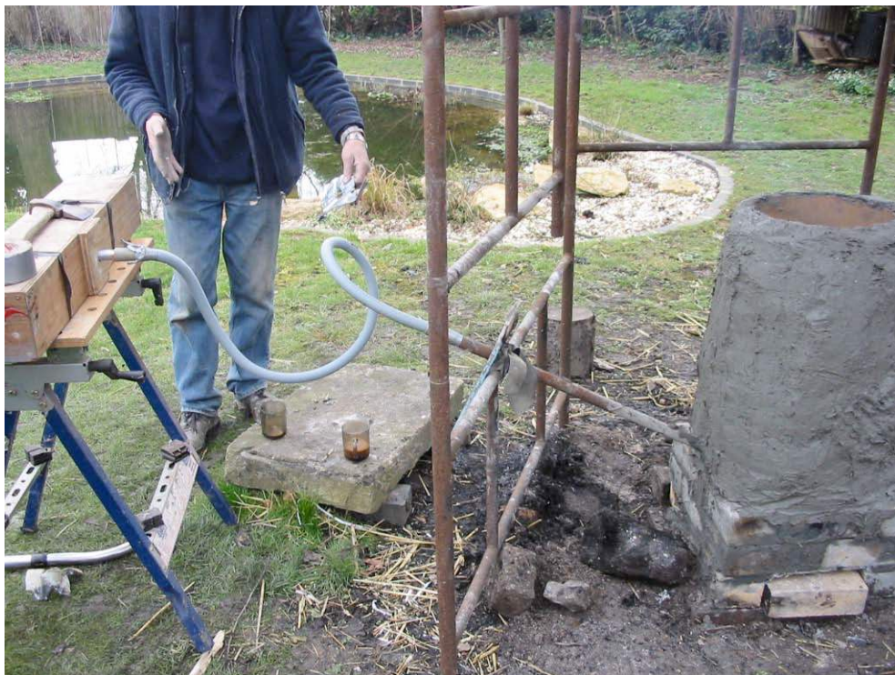
Chinese hand operated Box Bellows connected to Bloomery Furnace
