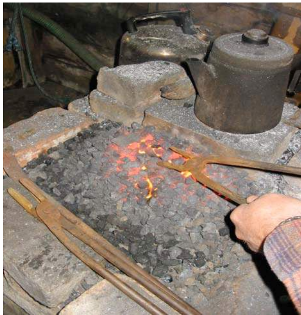
Heating the bloom in the forge
