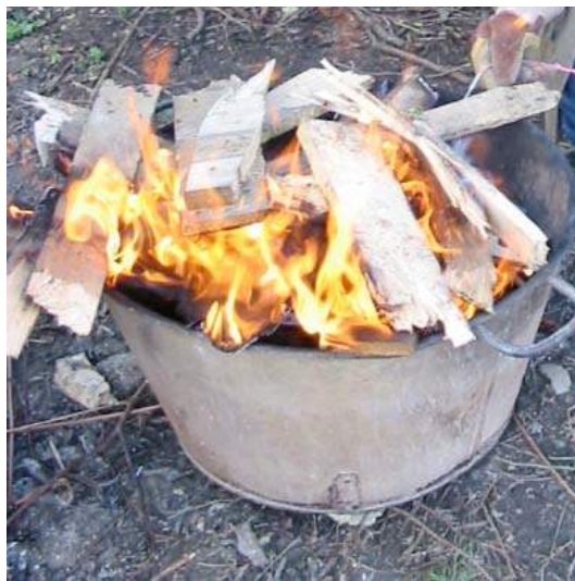
Roasting the iron ore in a metal bin
