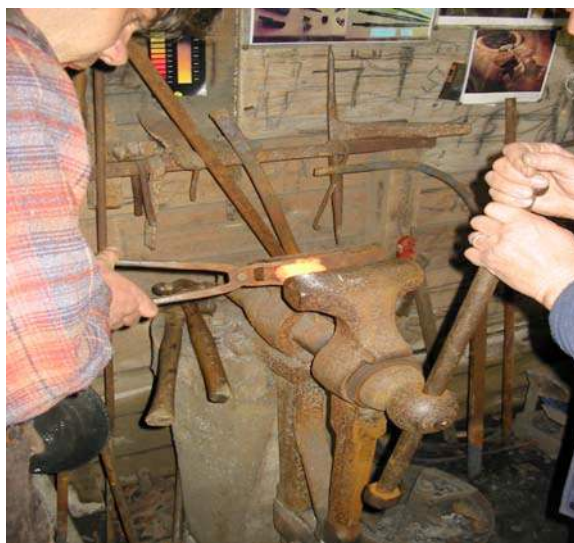
Squeezing the Bloom in a leg vice the bloom in the forge
