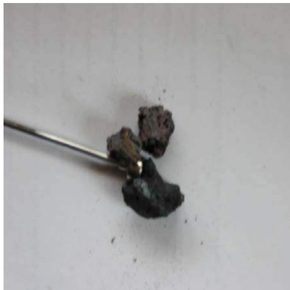
Roasted & Magnetised Iron
